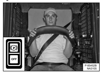
Lower the seat bar and engage the parking brake [Figure 128].
