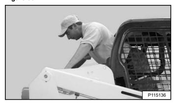
Exit through the rear of the operator cab [Figure 60].
