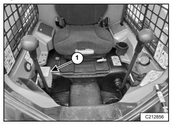
Move both steering levers toward the front of the operator cab and install a block (Item 1) **[Figure 185]** to hold the levers. Only one block is required to hold both steering levers forward.
