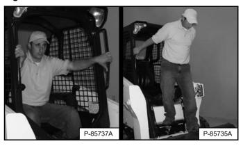
Exit the loader using grab handles, safety tread, and steps (maintaining a three-point contact) [Figure 139].
