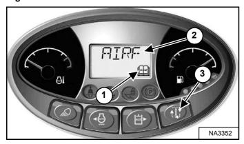
Replace the air filters only when necessary. The service indicator (Item 1) will FLASH. Press the Information button (Item 3) until the display screen shows the service codes. Service code [AIRF] (Replace Engine Air Filter) or [M0117] (Air Filter Plugged) will show in the display screen (Item 2) [Figure 206] when air filter replacement is necessary.
