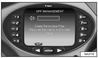
The machine will alert the operator when DPF service is required [Figure 260].
