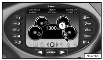
1. Press a scroll button repeatedly until the machine settings icon (Item 1) [Figure 48] is highlighted.
