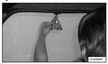
Pull on the tag on the top of the rear window to remove the rubber cord **[Figure 61]**.
