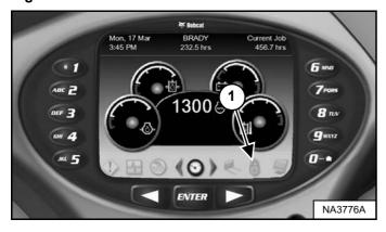
1. Press a scroll button repeatedly until the machine settings icon (Item 1) [Figure 36] is highlighted.
