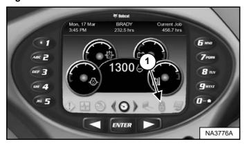
1. Press a scroll button repeatedly until the machine settings icon (Item 1) [Figure 40] is highlighted.
