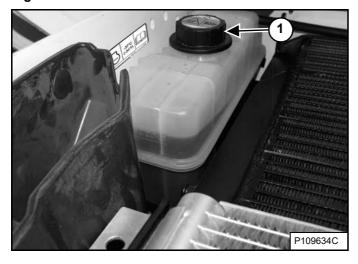
Remove the coolant fill cap (Item 1) [Figure 233].
