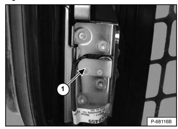
The cab door has a sensor (Item 1) [Figure 180] installed that deactivates the lift and tilt valves when the door is open.
