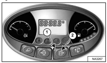
Press the Auxiliary Hydraulics button (Item 2) [Figure 106] once to activate the auxiliary hydraulics.
