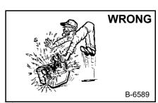
Lead-acid batteries produce flammable and explosive gases.
