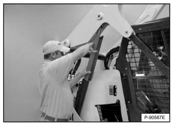
Have a second person remove the lift arm support **[Figure 174]** after the lift arms are all the way up.
