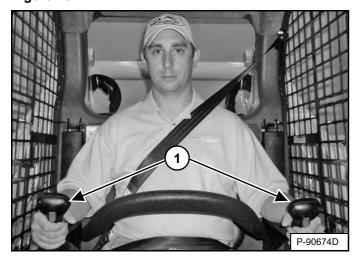
Both joysticks control drive and steering and are located on the left and right side in front of the seat (Item 1) [Figure 78].
