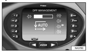
3. Press the [9] button to select inhibit mode [Figure 50].
