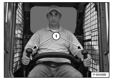
The steering levers (Item 1) **[Figure 72]** are on the left and right side in front of the seat.
