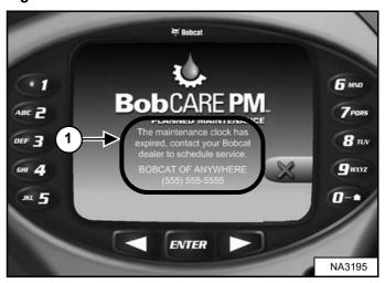
The Deluxe Instrumentation Panel will display a message (Item 1) **[Figure 303]** alerting the operator to service the machine.
