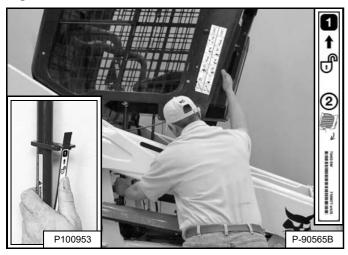
Pull down on the bottom of the operator cab until stopped by the latching mechanism [Figure 189].
