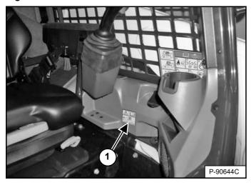
Inspect for damaged or missing back-up alarm decal (Item 1) [Figure 176]. Replace if required.
