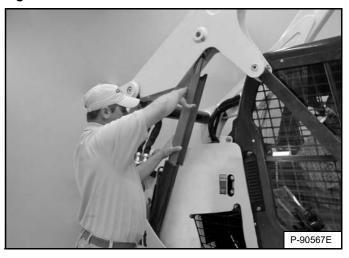
Have a second person install the lift arm support over the rod of one of the lift cylinders [Figure 172].
