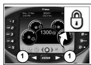
Press a scroll button (Item 1) repeatedly until the Machine Settings screen icon (Inset) is highlighted.
