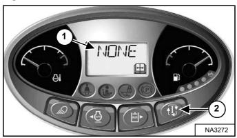
Press the Information button (Item 2) to cycle the data display (Item 1) **[Figure 299]** until the service code screen is displayed. If more than one service code is present, the codes will scroll on the data display.
