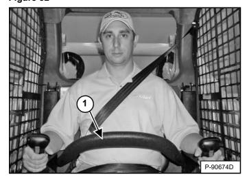
The Bobcat Interlock Control System (BICS™) has a pivoting seat bar with armrests (Item 1) [Figure 32]. The operator controls the use of the seat bar.
