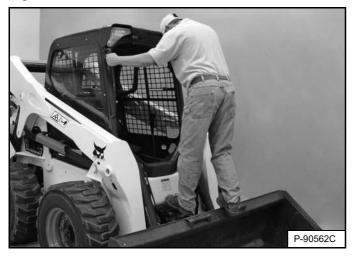
Use the bucket or attachment steps, grab handles, and safety treads (on the loader lift arms and frame) to get on and off the loader, maintaining a three-point contact at all times [Figure 120]. Do not jump.
