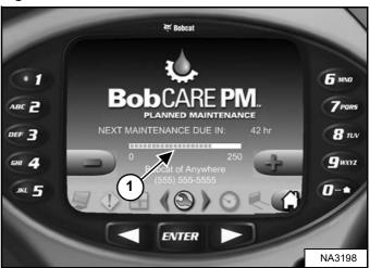
The Deluxe Instrumentation Panel will display a bar (Item 1) [Figure 304] showing the time remaining until next service. This bar will turn red when service is past due. [NEXT MAINTENANCE DUE] will change to [MAINTENANCE PAST DUE] and display the number of hours past due.
