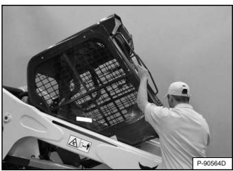
Lift on the grab handles and bottom of the operator cab [Figure 188] slowly until the operator cab is all the way up and the latching mechanism engages.
