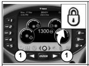
Press a scroll button (Item 1) repeatedly until the Machine Settings screen icon (Inset) is highlighted.
