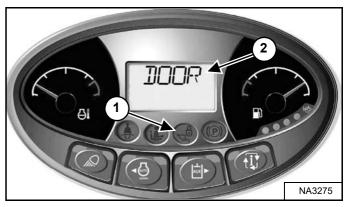
The LIFT AND TILT VALVE light (Item 1) **[Figure 181]** is OFF when the door is <u>closed</u>, the key switch is turned to RUN, the seat bar is lowered, and the PRESS TO OPERATE LOADER button is pressed.
