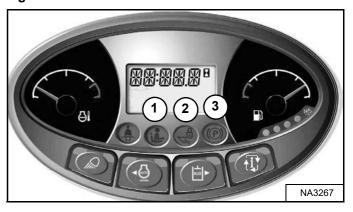
There are three display lights (Items 1, 2, and 3) **[Figure 33]** located on the left instrument panel that must be OFF to fully operate the machine.
