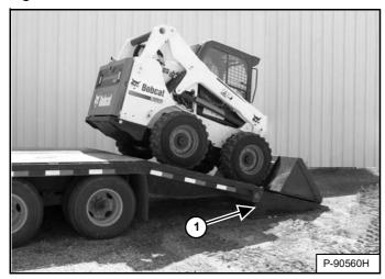
A loader with an empty bucket or no attachment must be loaded backward onto the transport vehicle [Figure 164].
