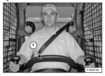
The seat bar restraint system has a pivoting seat bar with armrests (Item 1) [Figure 34].
