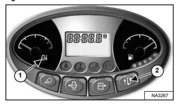
Frequently monitor the temperature and fuel gauges and BICS™ lights (all BICS™ lights must be OFF to operate loader) [Figure 136].
