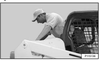
Exit through the rear of the operator cab [Figure 62].
